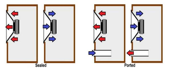
**Infinite** Loudspeaker Cabinets are completely sealed, so the air inside is trapped. As the cone moves back and forth it has to fight the internal air pressure, and energy is lost. Apart from that, this type of cabinet does have a particular type of compact punchy sound to it, and can be ideal for certain applications.
