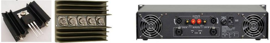
We need ventilation around a Power Amplifier to ensure the hot air coming off the heat sinks is blown away. Small fans are often built in to help us. If you cover the vents, or keep the Power Amplifier in a closed cupboard, or you work in some absurd summer heat (especially if the sun is shining directly onto the Amp) the power components will over-heat.
