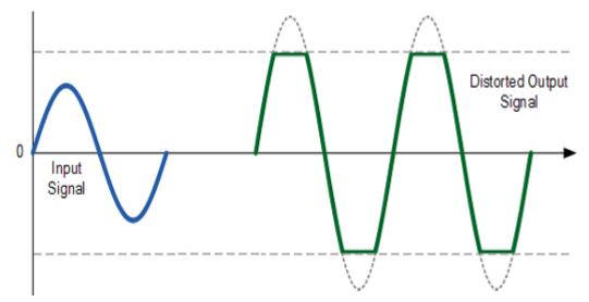
An Amplifier always has a **maximum voltage** that it can deliver. *This is determined by its design and its own power supply.* An Amplifier will also have a **maximum amplification** that it can deliver. *This is also determined by its design and its power supply.*
