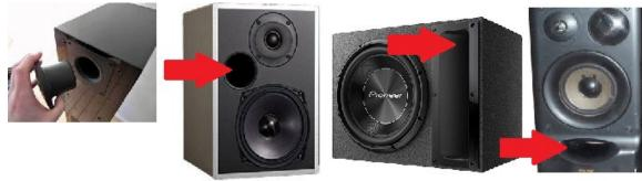
The "hole in the cabinet" developed over time, and a tube was added to the hole to make a resonant "Port". This tube resonates at a precise resonant frequency, which the manufacturer will choose to suit the cabinet.
