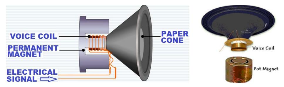
A cone loudspeaker takes advantage of the Dynamo effect. It has a short paper cylinder with a paper cone connected to it. A coil of wire is wrapped around the short cylinder, which is then suspended inside a magnet. Whenever we send an electrical (audio) signal through the coil it will generate magnetic fields which conflict with the magnetic fields of the pot-magnet (the dynamo effect), causing the tube and cone to vibrate back and forth in a similar manner to the electrical audio signal.
