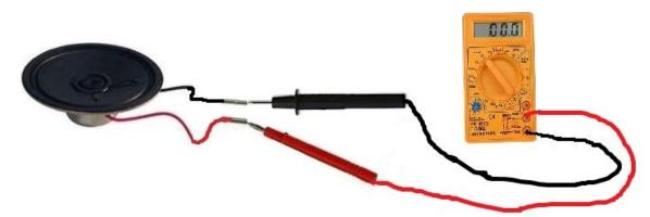
To measure the value of a Loudspeaker, you need to disconnect it first. Use a Tester (Multi-meter) set to read "*Resistance*" in ohms ( $\Omega$ ).
