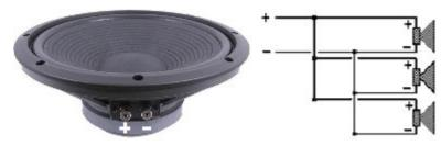
The voice coil on a loudspeaker may have a (+) sign to indicate which wire the signal should enter in to, and (-) to show the exit wire. The idea of this is to help you check that all cones in a cabinet are wired the same way (in-phase with each other). If one cone is pushing out while the other cones are pushing in (one is out-of-phase with the others) there will be a loss of power, and even a weird sound.
