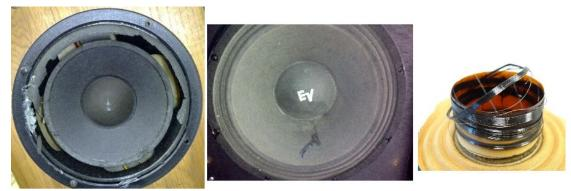
If a cone loudspeaker starts making a disgusting spluttering noise then you possibly have a tear in the paper cone, or a torn mount around the outer rim. If a cone loudspeaker stops working altogether then the fine copper wire in the voice coil may have melted (too much current caused by continuous loud volume is often the reason).
