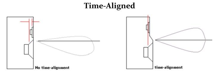
A Loudspeaker Cabinet has different sized cones moving at different speeds. The combined sound that results from this is slightly distorted. This is not a giant concern to people working in live environments, but for elite listening requirements there are cabinets constructed with the smaller cones further back.
