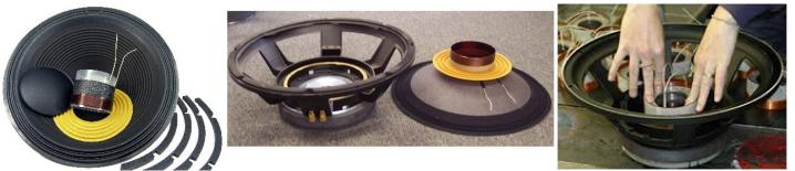
Simple tears on paper cones can be repaired with an appropriate rubber glue. Certain Loudspeaker Manufacturers sell replacement kits (a new paper cone and a new voice coil) but the kit needs to match the metal frame exactly.
